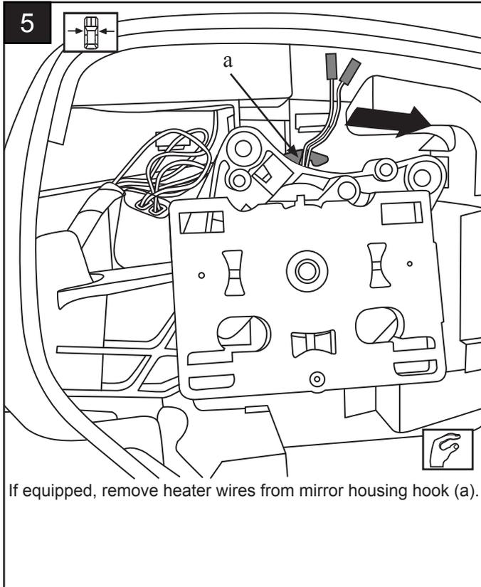
If equipped, remove heater wires from mirror housing hook (a).
