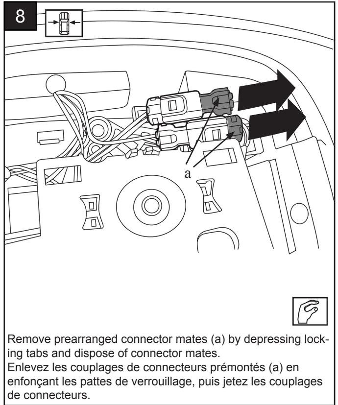
Remove prearranged connector mates (a) by depressing locking tabs and dispose of connector mates.
