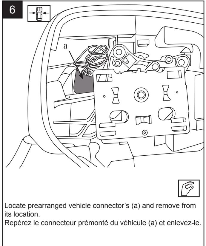
Locate prearranged vehicle connector's (a) and remove from its location.
